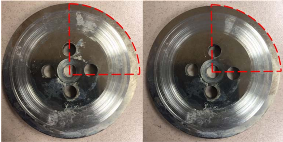
Figure 52. Tribofilm deposited on the surface of O1 stainless steel disk after testing in KCl polymer mud.
