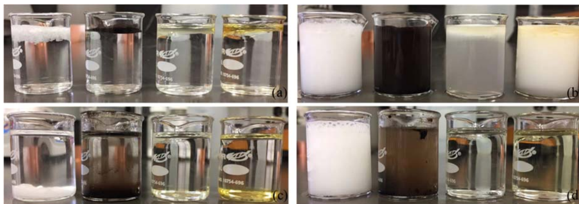
Figure 13. Solvability of additives in distilled water and base oil of OBM: (a) Distilled water with additives before mixing; (b) Distilled water with additives after mixing; (c) Base oil loaded with additives before mixing; (d) Base oil with additives after mixing. In all figures, the additives are Vikinol ® 18, 6010 ® , EvoLube ® G and Ultra Lube ® II, from left to right.
