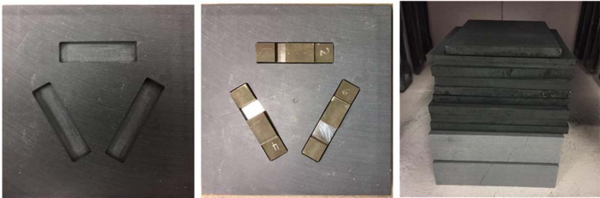
Figure 19. Experimental setup for self-welding behavior investigation of Inconel 617 ® and 800 HT ® .
