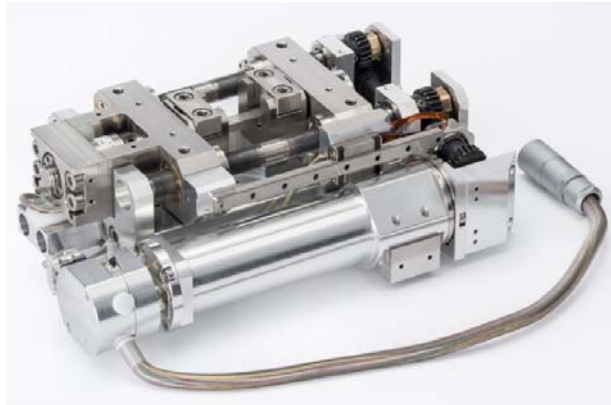
Figure 8. In-situ mechanical tensile stage for bonding strength measurements.
