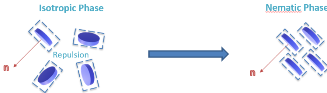
Figure 3. Isotropic-Nematic phase transition in calamitic particles. The isotropic phase occurs at low concentrations and lacks any form of order with high orientational entropy. The nematic phase forms at higher concentration and favors translational entropy.
