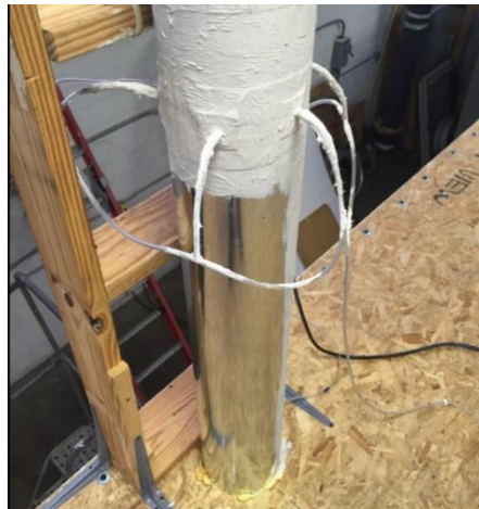
Figure 17: Five sampling points across exhaust duct
