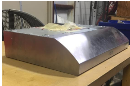
Figure 47: Typical under the cabinet (UTC) range hood analyzed in discharge orientation study
