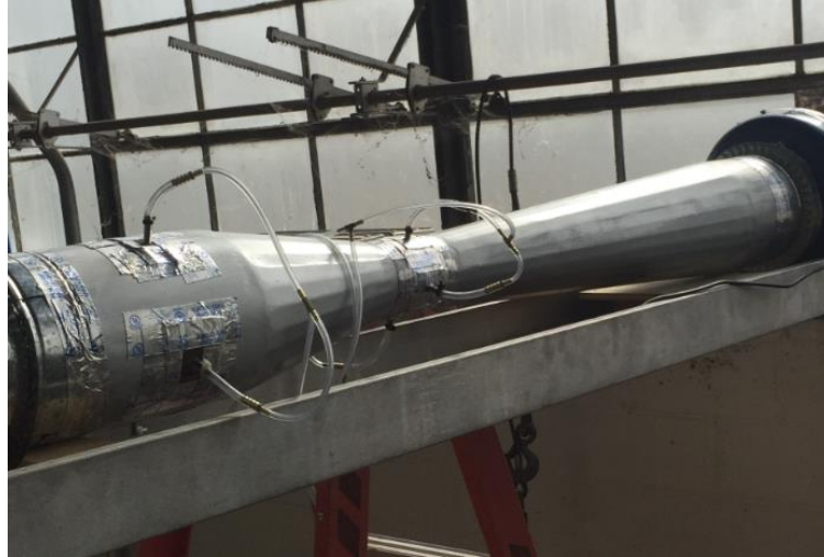
Figure 7: Venturi tube used for flow measurement
