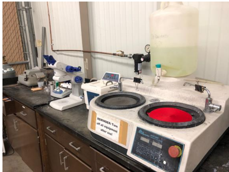
Figure 4. Mechanical polishing apparatus used for sample preparation.
