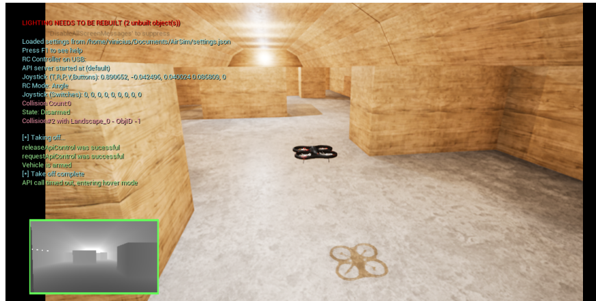
Figure 7.4: Warehouse scenario created for the collision avoidance task using Unreal Engine for visually realistic textures and objects. Reprinted from [7].
