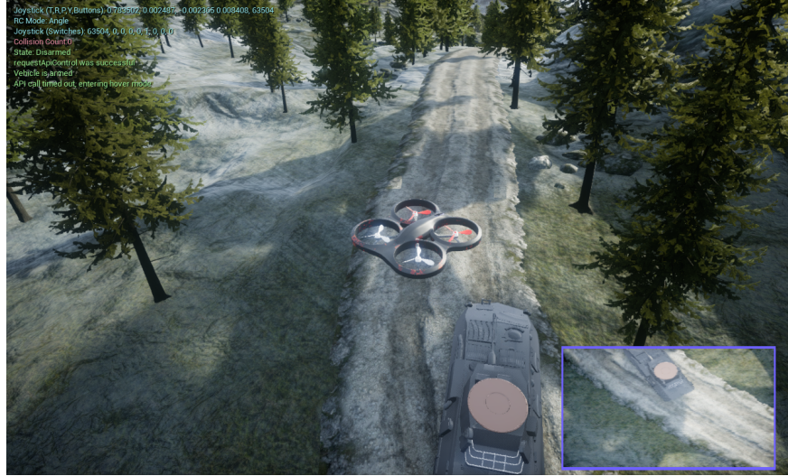
Figure 9.3: Screenshot of AirSim environment and landing task. Inset image in lower right corner: downward-facing camera view used for extracting the position and radius of the landing pad which is part of the observation-space that the agent learns from. Reprinted from [8].
