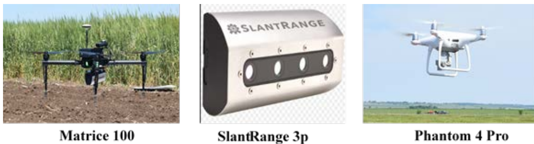
Figure 18. Unmanned Aerial System (UAS) platforms and sensors used in this study. Matrice 100 was used to carry SlantRange 3p (multispectral sensor).
