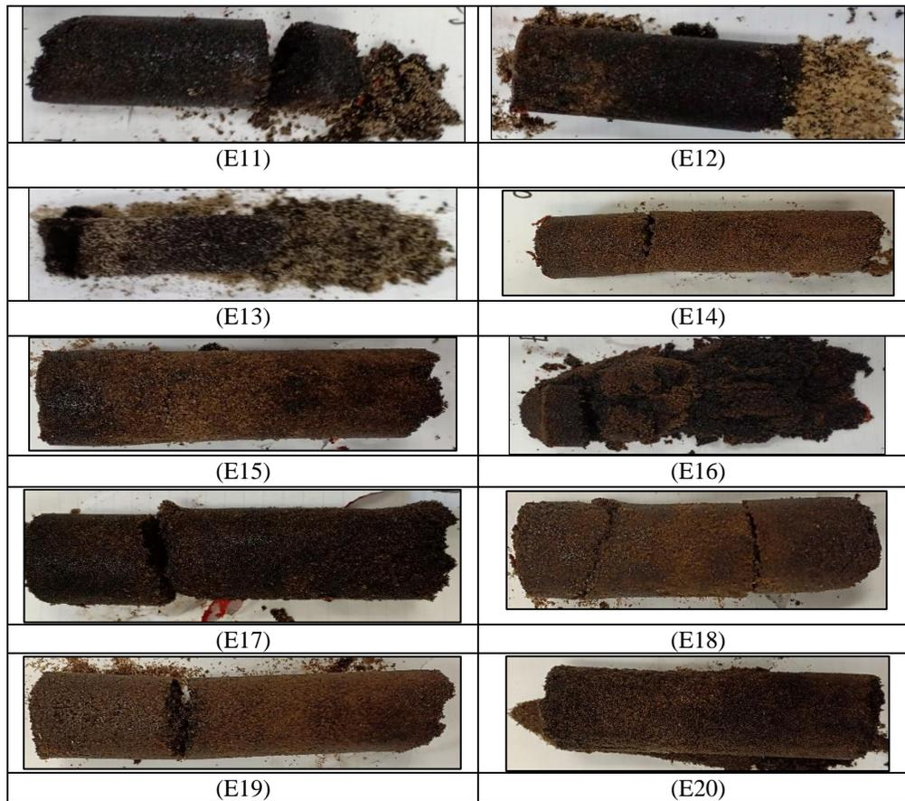
**Figure 4.20—Spent rock images for all experiments conducted with Oil 2. Injection is from left (inlet) to right (outlet). For experiment naming, refer to Table 3.2.**
