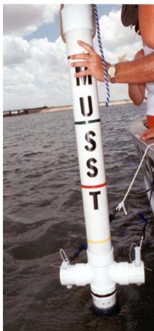
Figure 3. Multiple Underwater Syringe Sampling Tool (MUSST).
