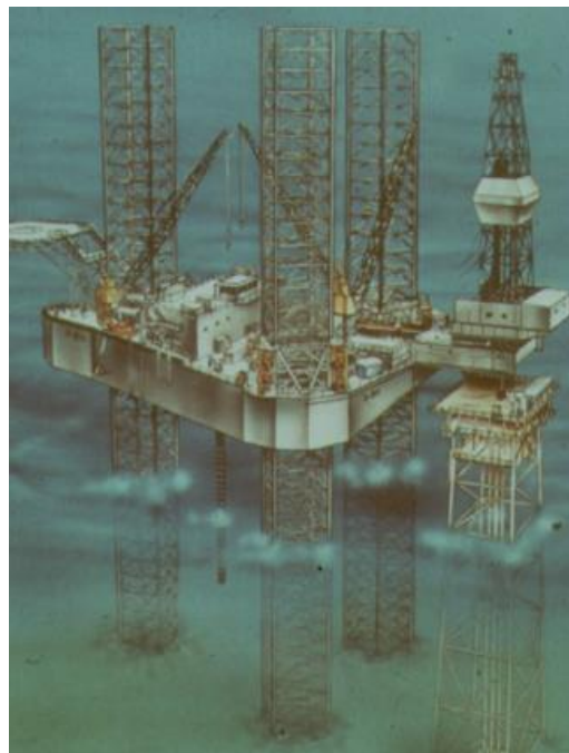
Figure 1.4 Jack-up platform, courtesy of Dr. Aubeny.
