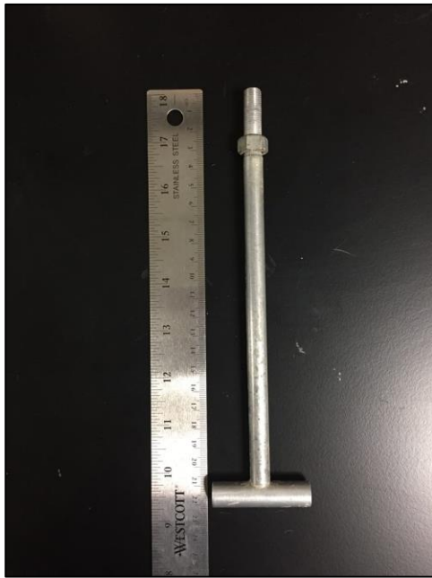
Figure 2.11 Full-flow penetrometer, T-bar penetrometer model.
