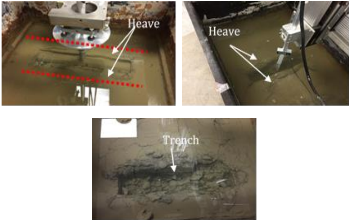
Figure 6.7 Some photos show the heave and the formed trenches.
