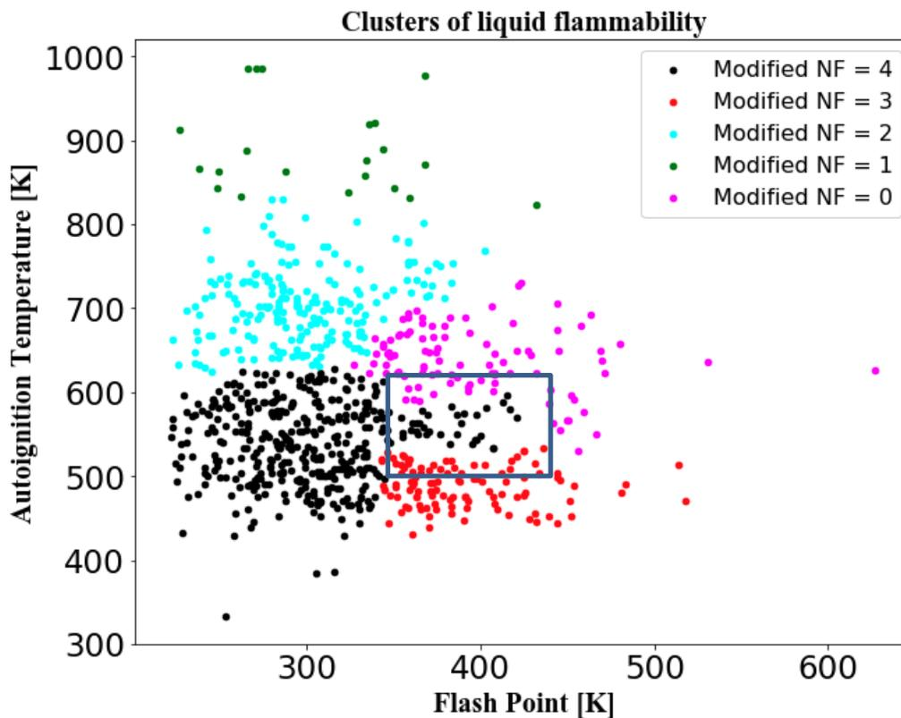
**Figure 12.** Clusters of liquid flammability using HC algorithm
