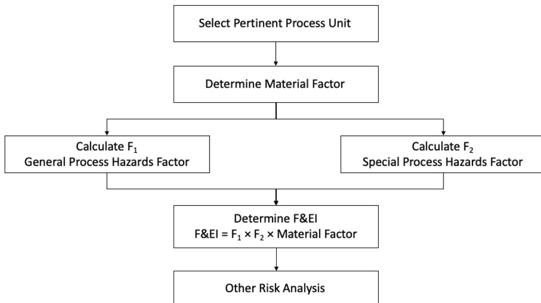
**Figure 2.** Procedure for calculating Dow's F&EI
