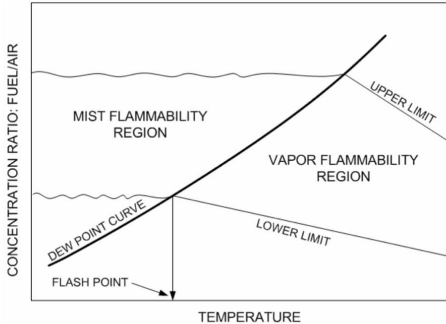
**Figure 5.** Schematic flammability diagram at constant pressure [32]
