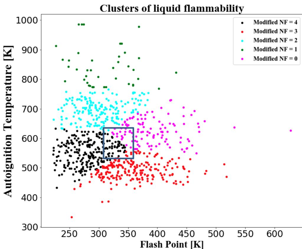
**Figure 10.** Clusters of liquid flammability using KC algorithm
