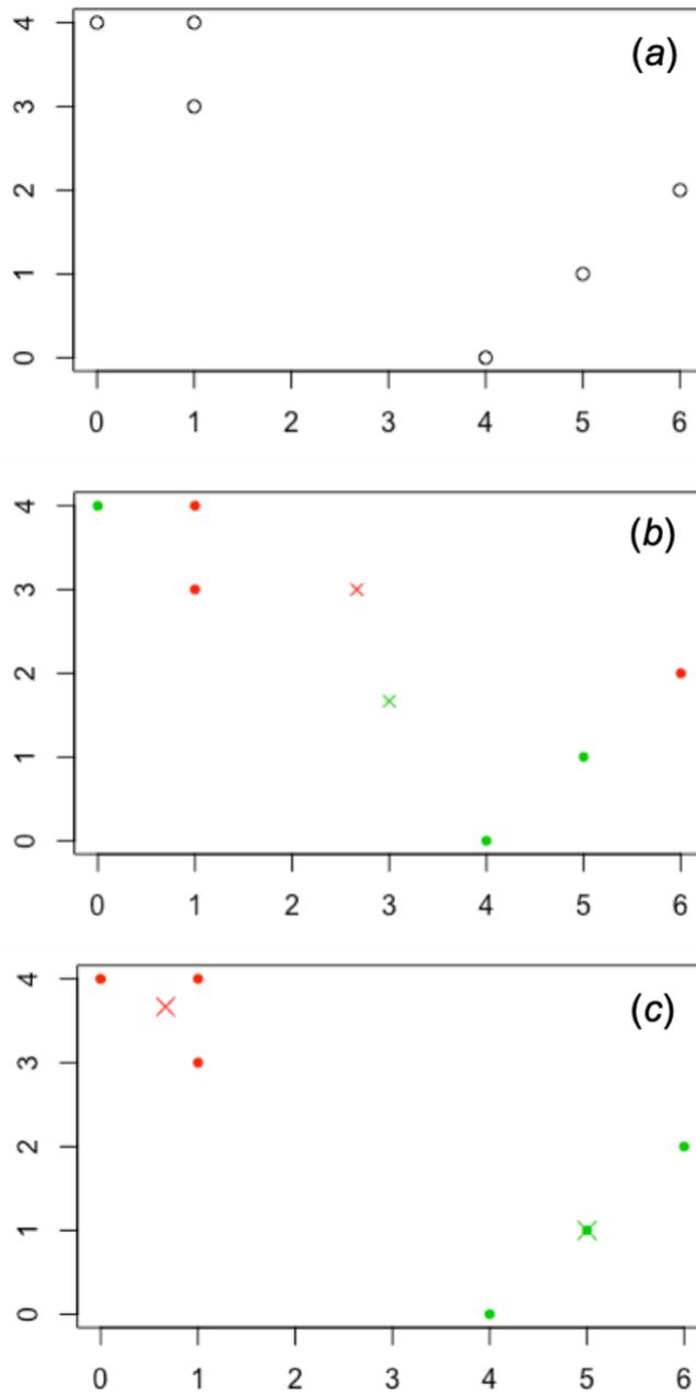
**Figure 3.** K-Mean clustering explanation: (a) Unclassified raw data; (b) Random classified data points and centroids; (c) Local optimal classification
