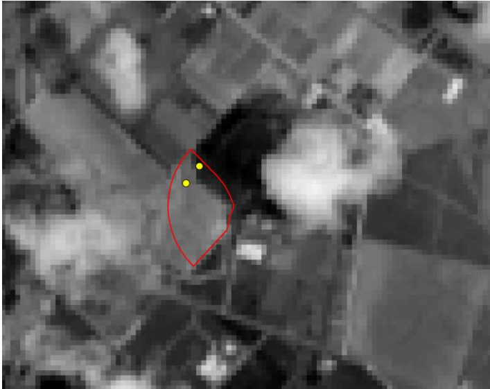
Fig. A1. Landsat 8 near-infrared (NIR) image (30 m pixel resolution) over study area (red outline) on June 16, 2017. The two yellow circles refer to the eddy covariance flux towers (Tower A and Tower B) shown in Figure 1. Note that the upper flux tower (Tower A, Fig. 1) is located within cloud shadows from a scattered cloud located east of the field. Therefore, all SAT analysis was focused over pixels that do not contain clouds and/or cloud shadows.
