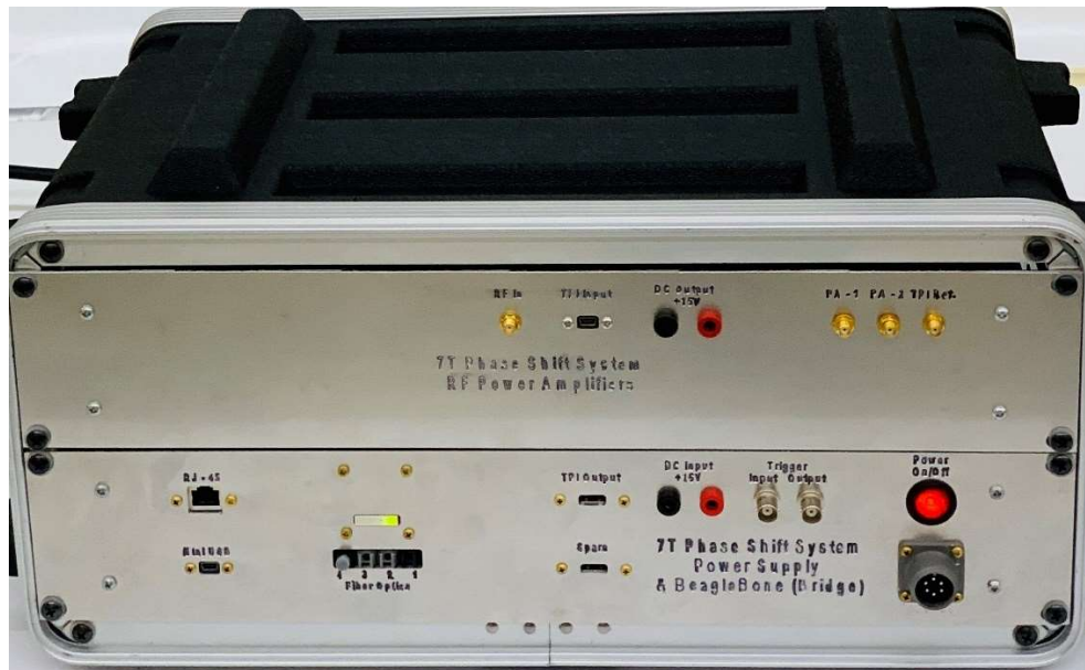
Figure 3.7 – Power Supply Unit & BeagleBone(Bridge)/ RF Amplifier Unit
