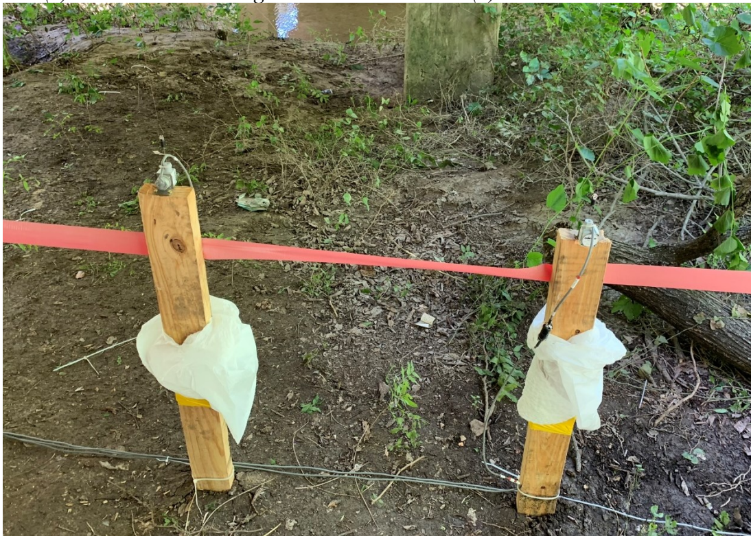
(c) Installed String Potentiometers
