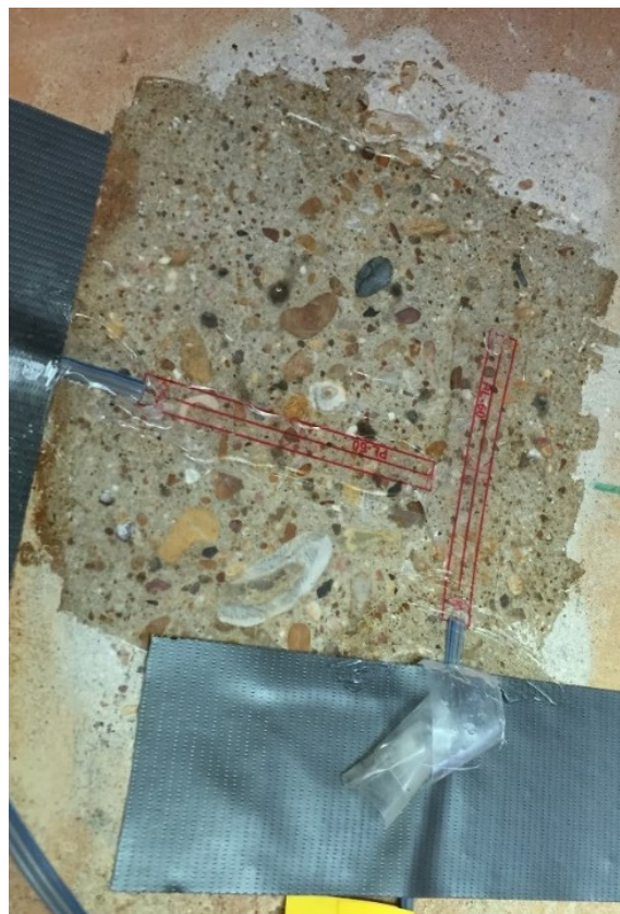
Figure 7.8. Close-Up of Strain Gauge Installation
