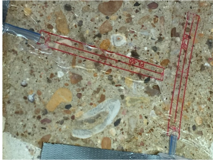
(b) Tokyo Measuring Instruments Lab PL-60-11-3LJCT Strain Gauges
