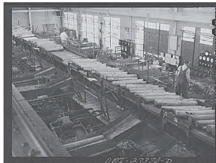
Lufkin, Texas. Southland Paper Mill. Grinding room where pulp logs are made into ground wood.
