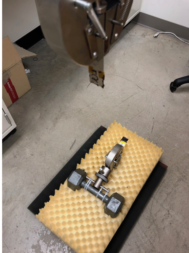
Figure 3.13: Green strength test for the 2 min RF lap shear sample, the sample failed after a few seconds of having the weight applied
