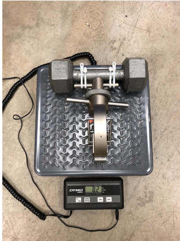
Figure 3.12: Weight and tensile grip mass measured at 8.2 kg, used for the green strength test in this study
