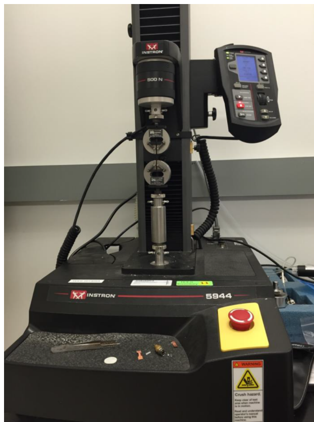
Figure 2.25: Instron 5944 load frame used for tensile and tear tests.
