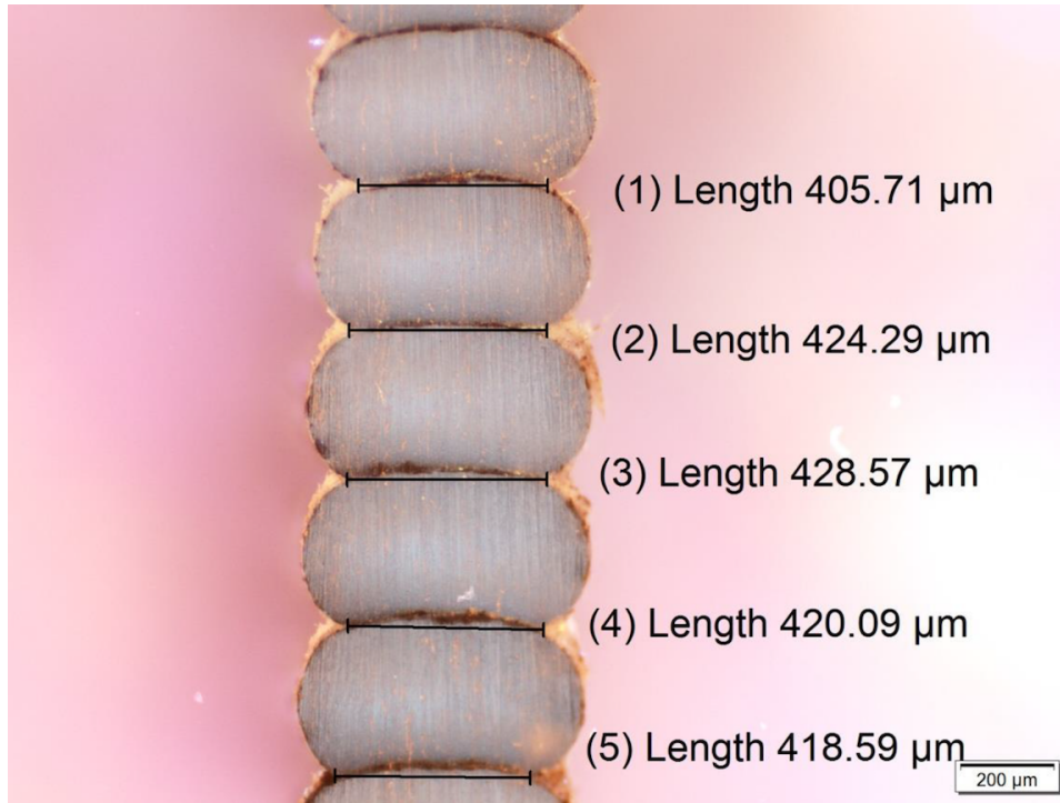
Figure 2.27: Optical microscope image of a tear test sample viewed edge-on to determine the mean weld line thickness.
