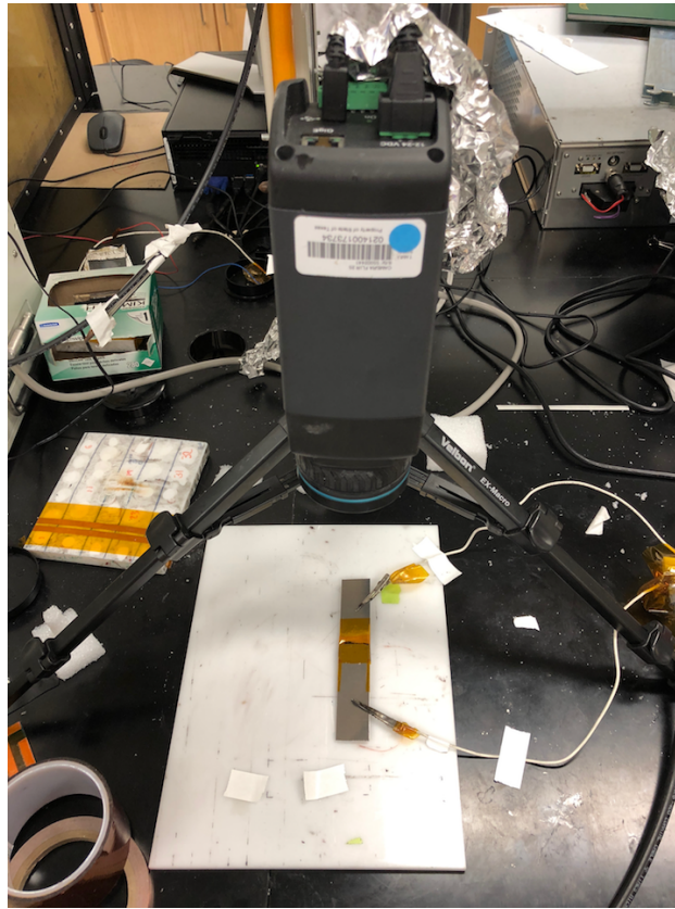
Figure 3.10: Setup for monitoring lap shear temperature with FLIR camera.
