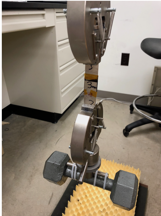
Figure 3.14: Green strength test for the 3 min RF lap shear sample, the sample held the weight for approximately 30 min without failing
