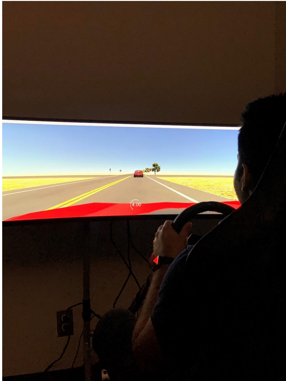
Figure 46. Image of the Participant Following the Leading Vehicle on the Driving Simulator
