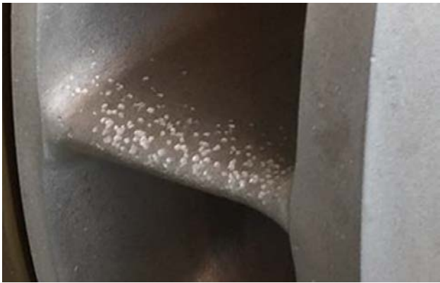
Figure 9. Evidence of erosion on suction surface of expander wheel.
