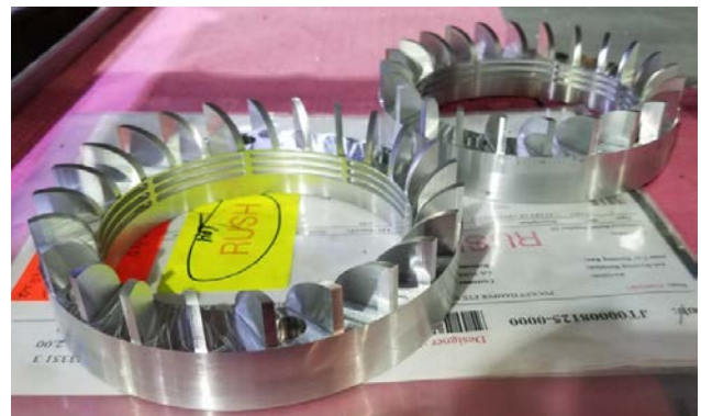
Figure 22. Redesigned front wheel seals.
