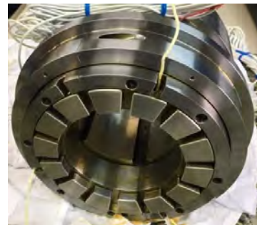
Figure 42: Thrust Bearing with Strain Gauge
