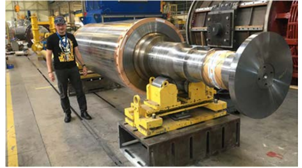
Figure 53 – 80 MW/4000 rpm Shaftless Induction Rotor
