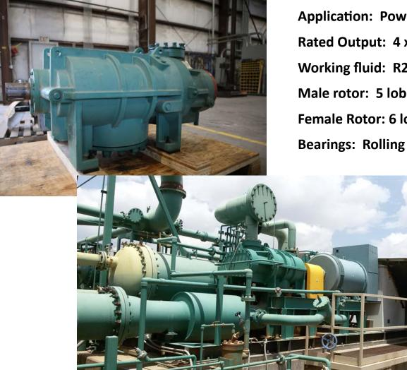
Application: Power generation Rated Output: 4 x 1,000 kW (4 identical units installed) Working fluid: R245fa (refrigerant) Male rotor: 5 lobes (1800 RPM) Female Rotor: 6 lobes (1500 RPM) Bearings: Rolling element (cylindrical and tapered)
