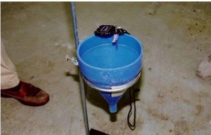
Figure 5: Fill Flow Cone to the Specified Level and have Stopwatch Ready
