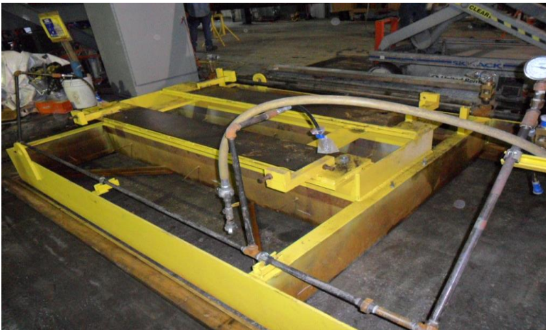
Figure 18: Example of Skid Mounted Equipment
