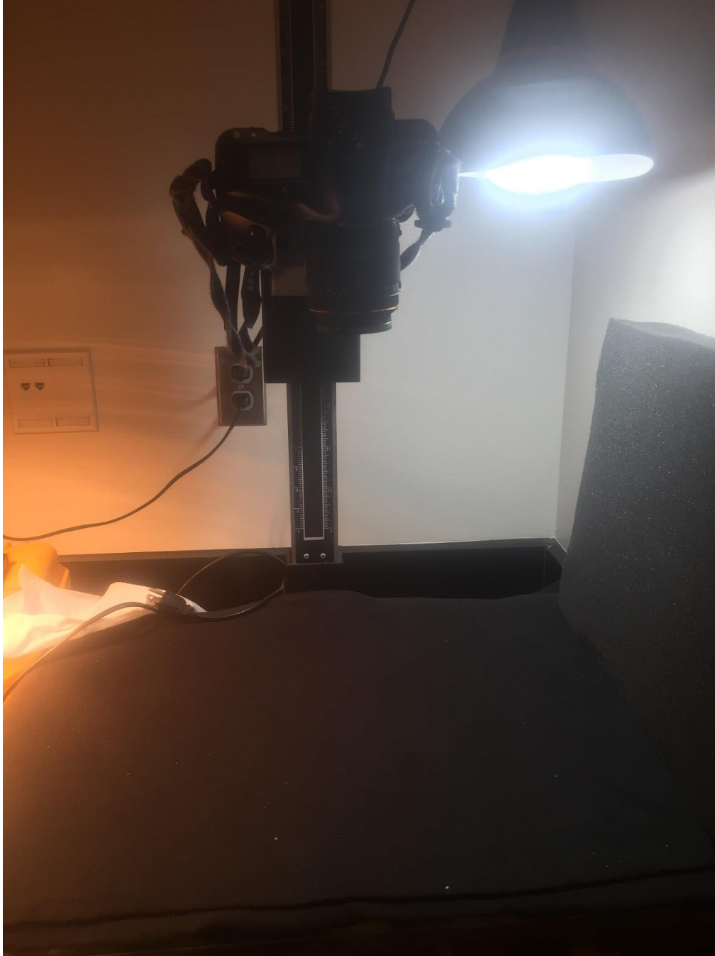
Appendix 4: Copy stand apparatus for photographing the snails
