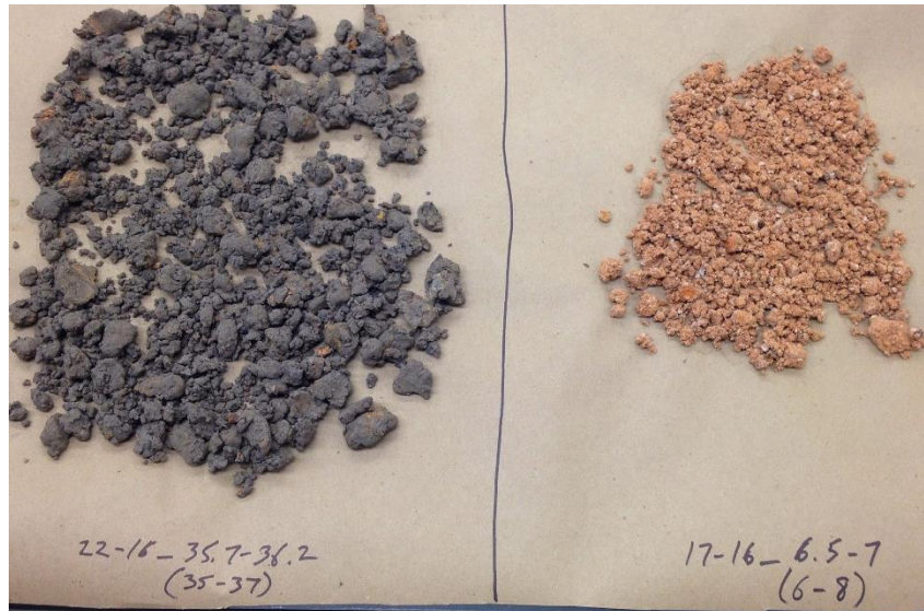
Figure 1. Drying samples showing common reduced (L) and oxidized (R) mineral conditions.
