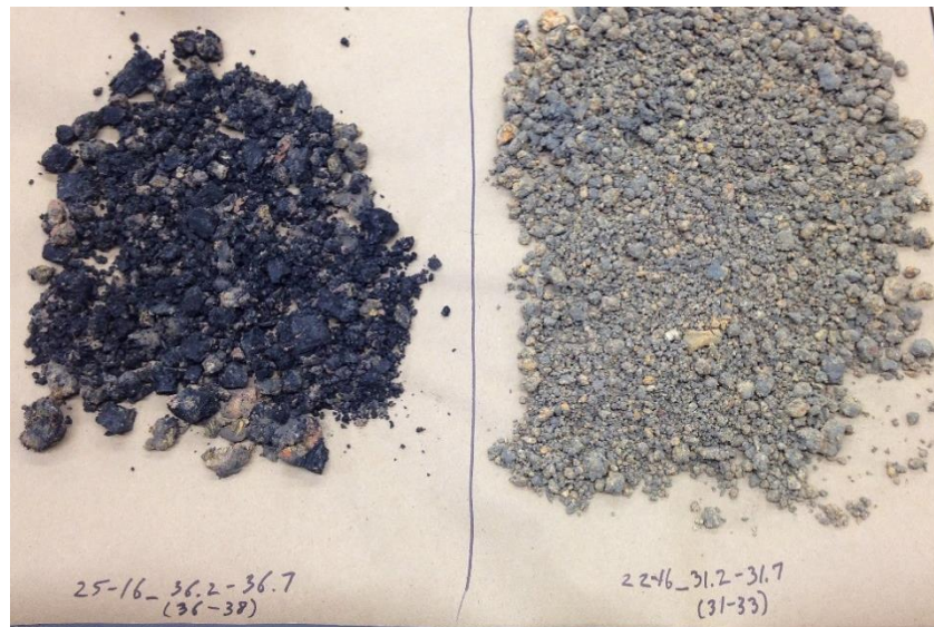
Figure 2. Drying samples showing colorations due to lignite (L) and partial oxidation (R).
