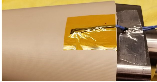
Figure 4.10: Photograph of upstream mounting holes with transducers installed and cables secured using Kapton tape.
