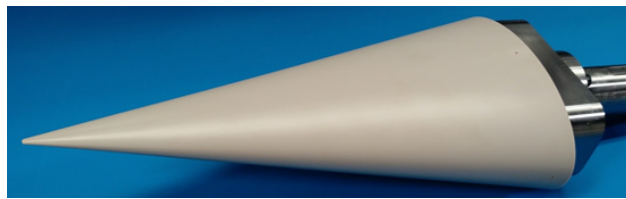
Figure 4.4: Improved 38.1% scale PEEK elliptic cone model.
