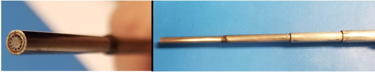
Figure 3.7: Photograph of XCEL-100-5A pressure transducer in pitot configuration. Screen shown at left and probe construction at right.
