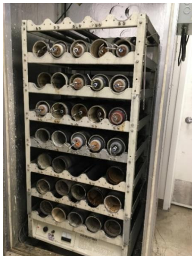
Figure 2-4 Thermostatic incubator equipped with horizontal roller.
