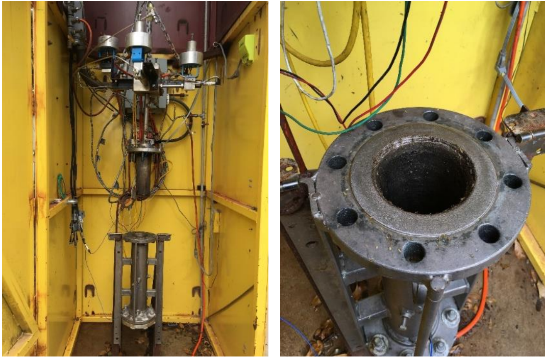
Figure F-1 Shock tube apparatus (left) and its biomass inlet (right).
