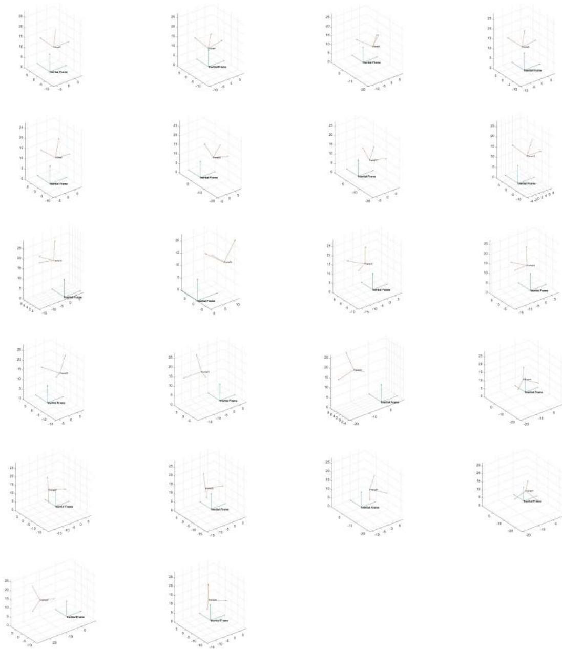
Figure D.1: Extrinsic Projections as computed using the Homography optimization algorithm corresponding to each image plane projection shown in Figure 6.2 for Dataset 1. The distances are provided in inches. Brown's distortion is employed in the optimization process. The frames are ordered from the top left to the bottom right.
