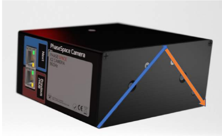
Figure 3.3: The direction of increasing position values for both detectors is shown, as inferred from Table 3.1. The orange arrow shows the direction of increasing position values for Detector 0 and the blue line shows the direction of increasing position values for Detector 1
