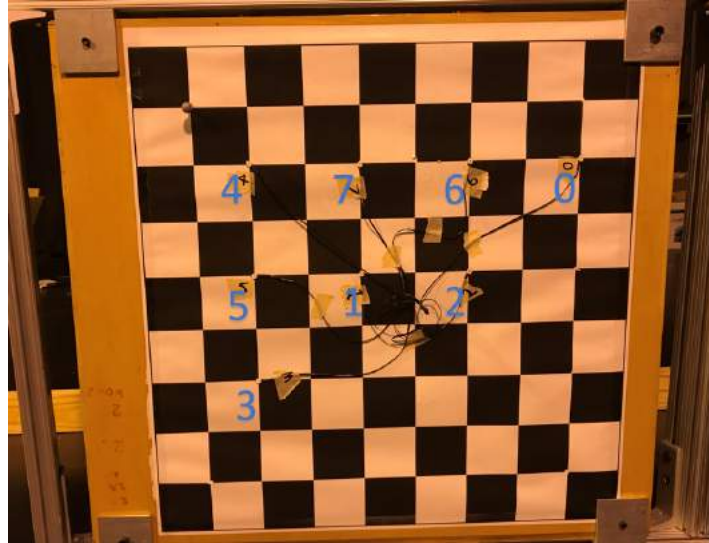
Figure 3.2: The beacon arrangement on the checkerboard pattern is shown. The number next to each beacon denotes its assigned reference number in the Phasespace SDK
