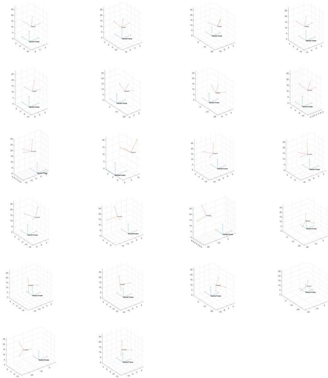
Figure D.2: Extrinsic Projections as computed using the Homography optimization algorithm corresponding to each image plane projection shown in Figure 6.2 for Dataset 1. The distances are provided in inches. Geometric distortion is employed in the optimization process. The frames are ordered from the top left to the bottom right.
