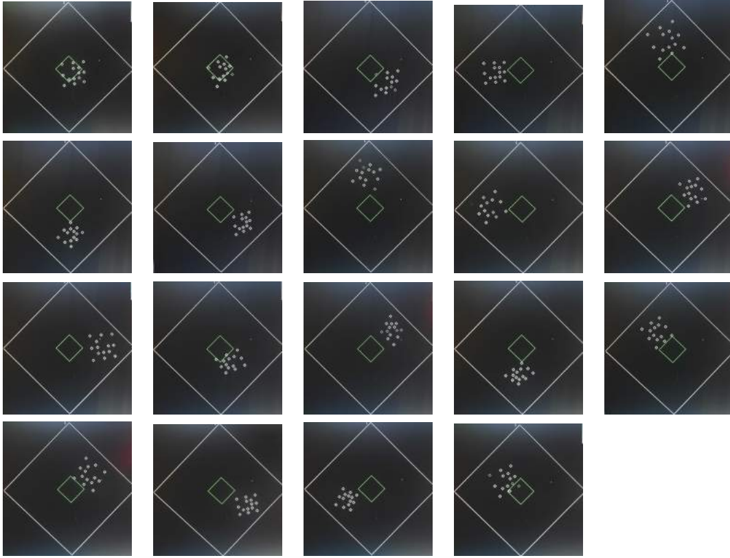
Figure 6.17: Image plane projections of each pose of the board as seen through the Phasespace Viewer. The frames are ordered from the top left to the bottom right.
