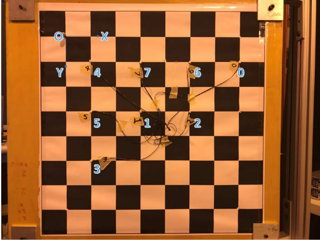
Figure 3.4: The inertial coordinate system with beacon positions. "O" is the origin and "OX" and "OY" represent the inertial planar axes.
