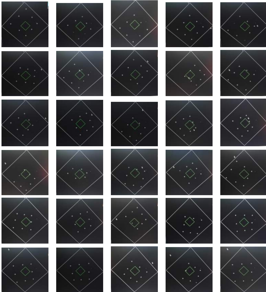
Figure 6.2: Image plane projections of each pose of the board as seen through the Phasespace Viewer. The frames are ordered from the top left to the bottom right.
