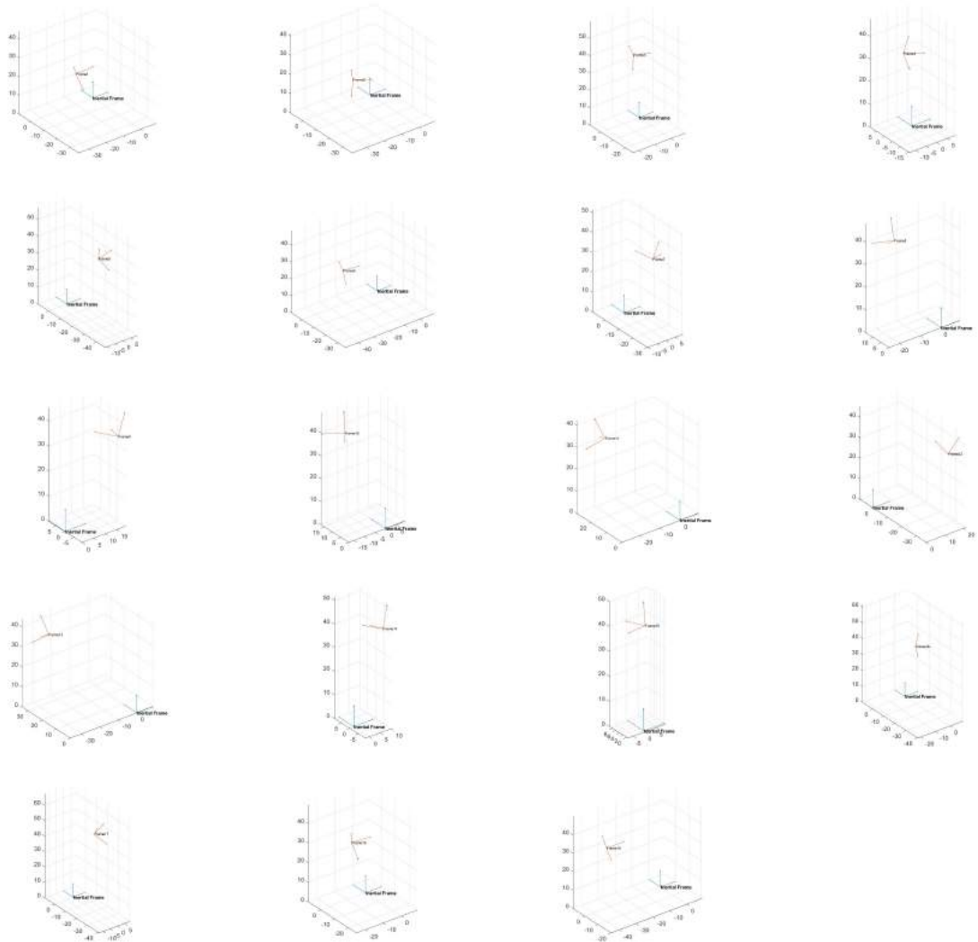
Figure D.5: Extrinsic Projections as computed using the Homography optimization algorithm corresponding to each image plane projection shown in Figure 6.17 for Dataset 3. The distances are provided in inches. Brown's distortion is employed in the optimization process. The frames are ordered from the top left to the bottom right.
