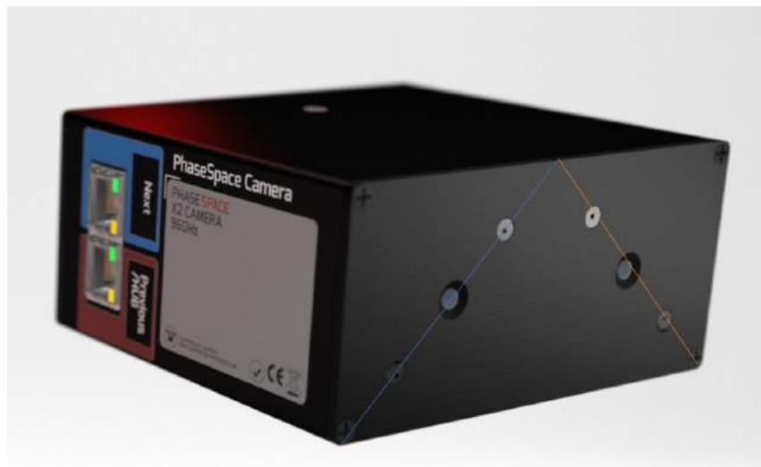
Figure 3.1: The orientation of the two linear detectors in the Phasespace camera is shown. The orange line represents detector 0 and blue line represents detector 1. Original image taken from [2]
