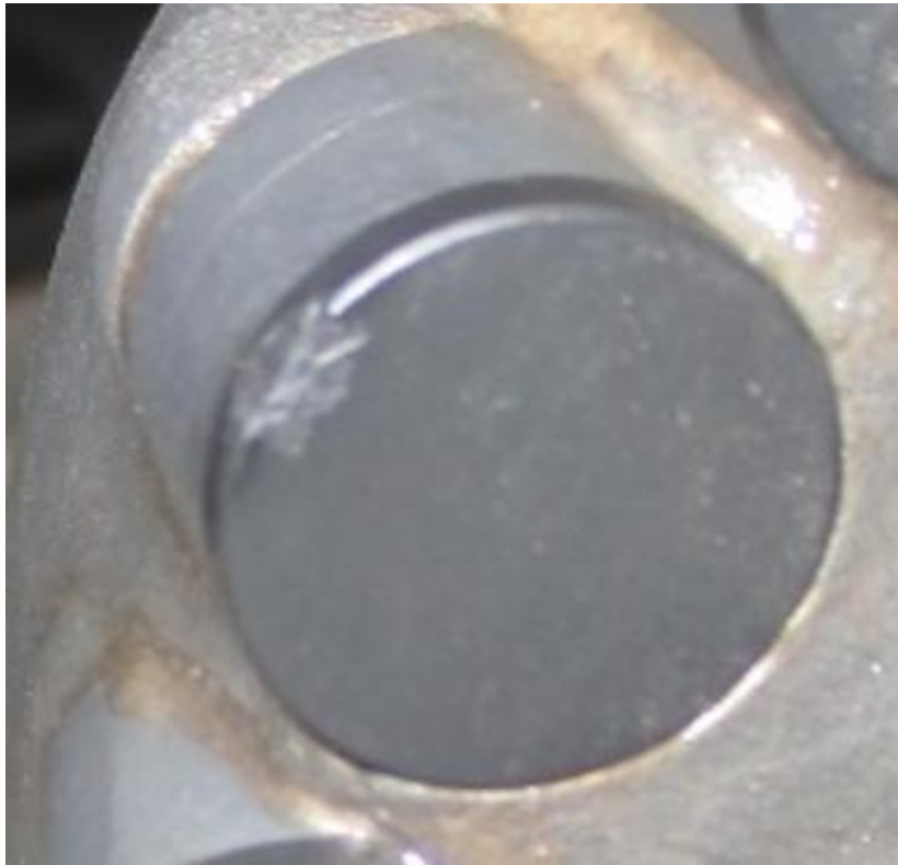
Fig. 6.4 – Thermal damage starting on PDC cutter (Courtesy of Ultra Petroleum)
