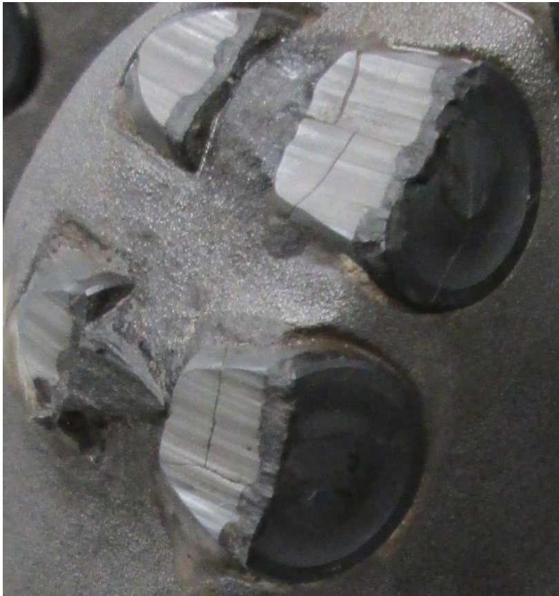
Fig. 6.3 – Close up of thermal wear and degradation on PDC cutters from Well 2 (Courtesy of Ultra Petroleum)
