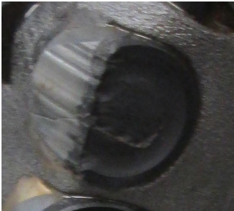
Fig. 6.2 – Close up of lateral impact damage
