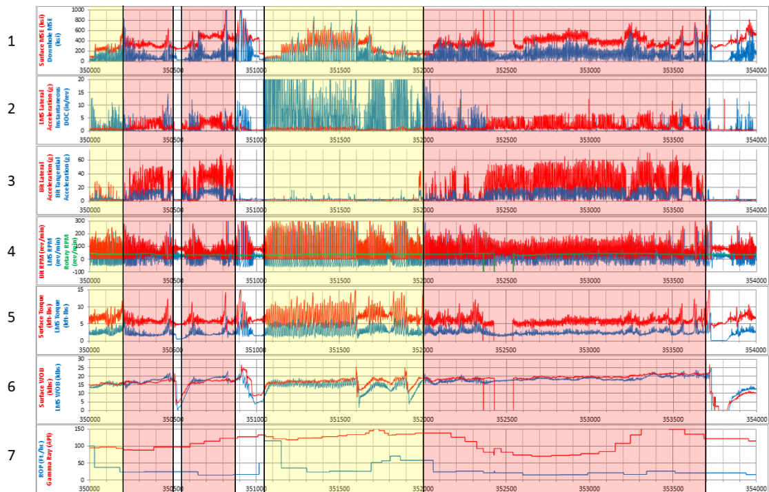
Fig. 5.1 – Surface and downhole measurements versus time Well 1 Bit Run 2
