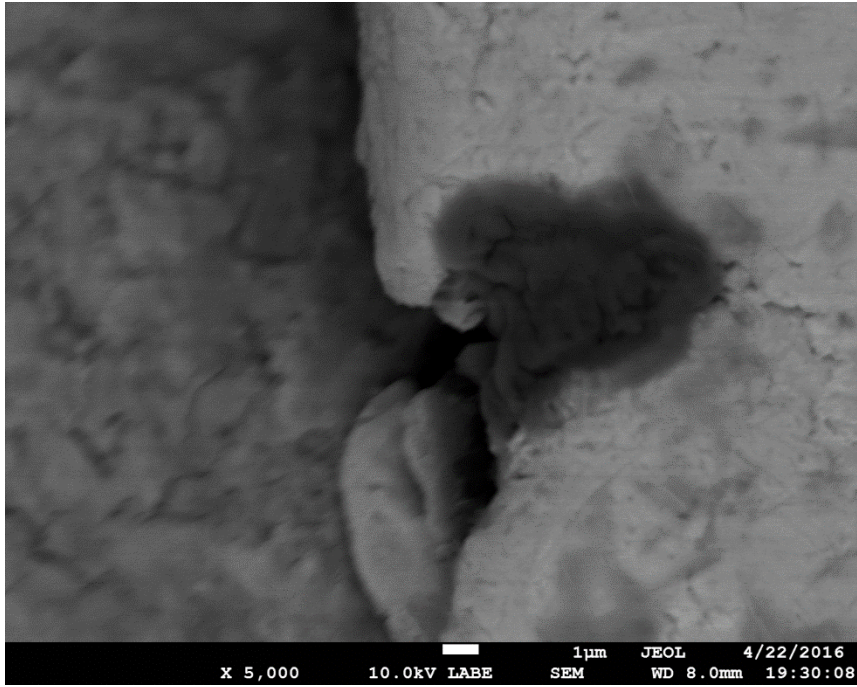
Figure 27: Flaw on titanium substrate surface infiltrated by geopolymer gel
