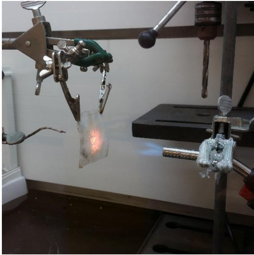
Figure 5: Flame testing of a fire retardant geopolymer coating
