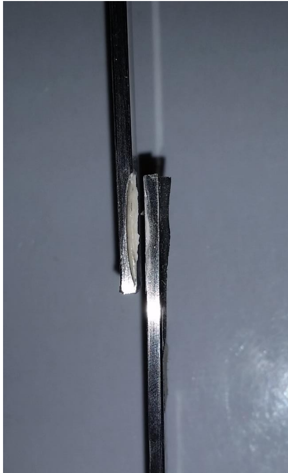
Figure 14: Shear test specimen after shear failure
