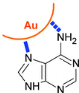
Figure 10. Chemical structure and assumed orientation of the nucleotide adenine on gold 735\text{ cm}^{-1} peak from the 100 nM chip was difficult to distinguish from the noise.
