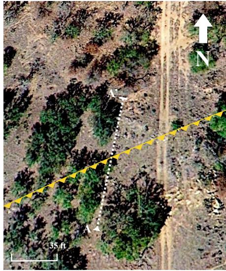
Figure 6.7: Shows the location of a high-angle fault traversed by the GPR line A to A'. The line was acquired in the northward direction while the fault dips to the south-east.
