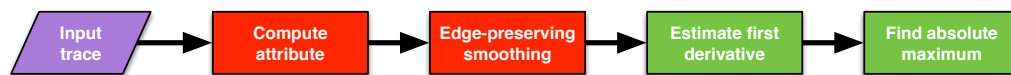
Figure 4.18: Automatic first-arrival picking workflow. Processes colored in red indicate steps that differ from Coppen's method.
