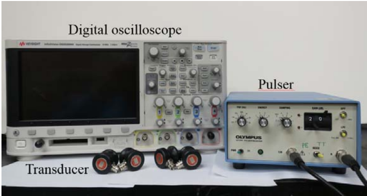
Figure 2.2 Equipment used for acoustic measurement - pulser, ultrasonic transducers, and the digital oscilloscope.
