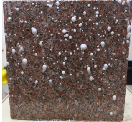
Figure 3.10 Comparison of bubble leakage before and after the first stimulation (Face 4, granite Specimen#2).
