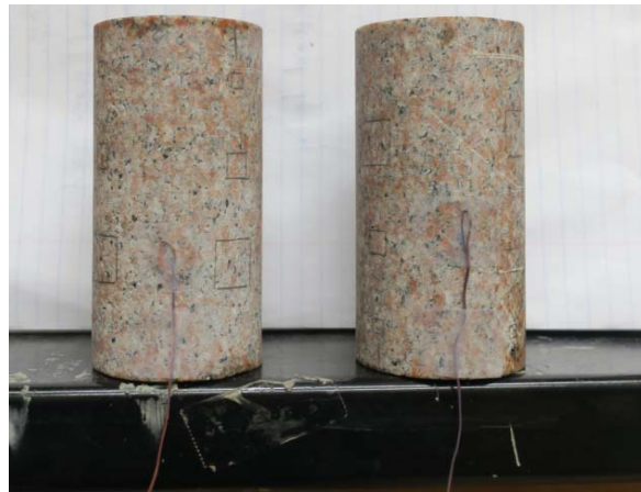
Figure 4.3 Thermocouples attached on core specimen with glue - the glue cured for 12 hours before starting to heat (Granite Core Specimen #1 and Specimen #2).
