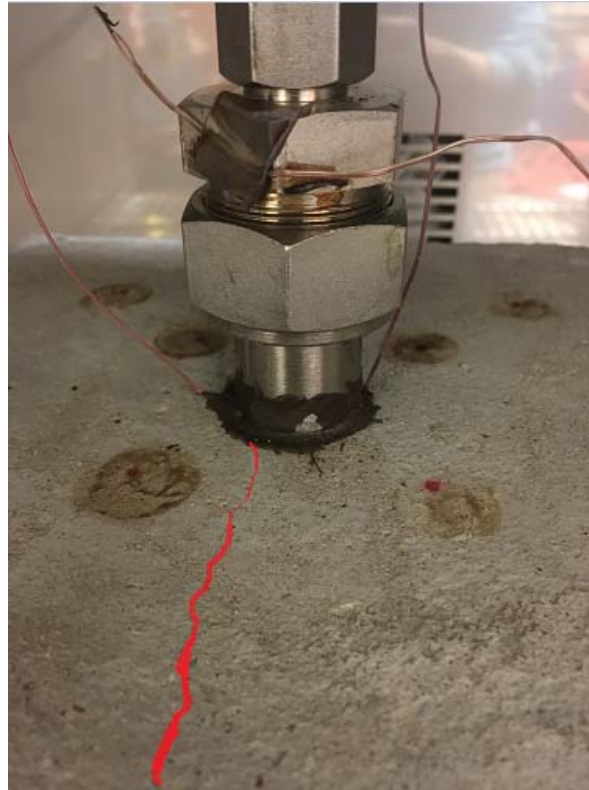
Figure 2.30 “Short-cut” fractures initiate from the borehole and propagate to the top surface (Specimen 14).
