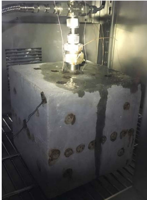
Figure 2.32 Water bubble indications during pressure decay tests (Specimen #18).
