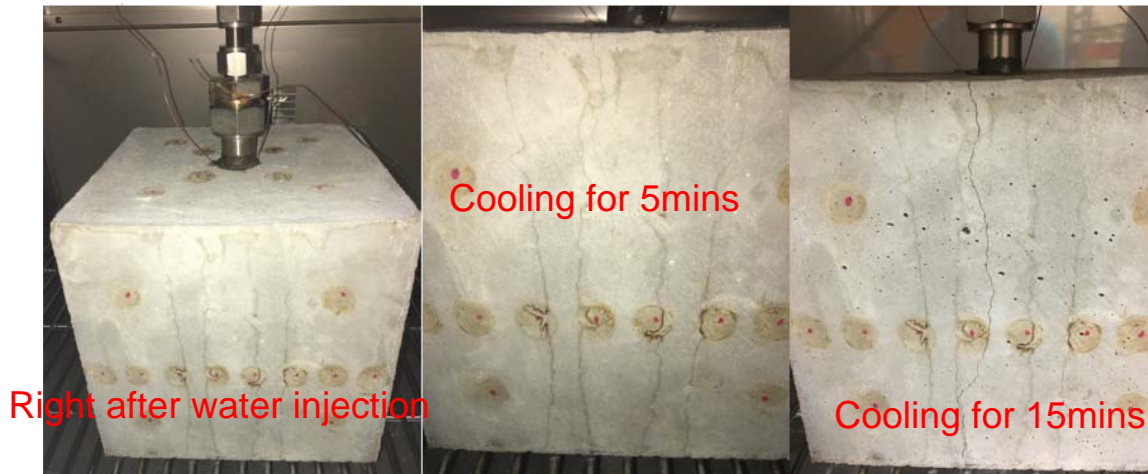
Figure 2.35 Fractures propagated and widened during the cooling period (Specimen 14) (oven door kept open during cooling).
