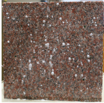
Figure 3.9 Comparison of bubble leakage before and after the first stimulation (Face 2, granite Specimen#2).
