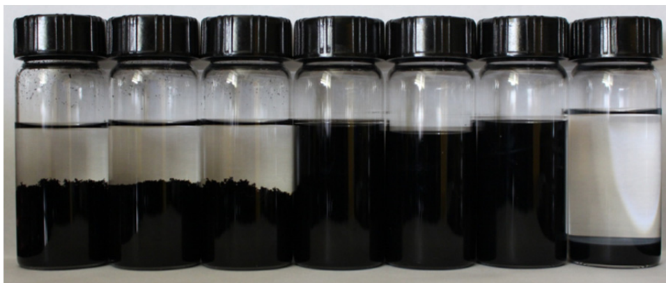
Figure 39. Photograph of MWCNTs dispersion in methanol with different concentrations of ZnO nanoparticles (MWCNTs concentration: 0.2 mg/mL) after 3 months. From left to right, the weight ratio of ZnO:MWCNT equals to 0:1, 1:2, 1:1, 2:1, 4:1, 8:1, and 20:1.
