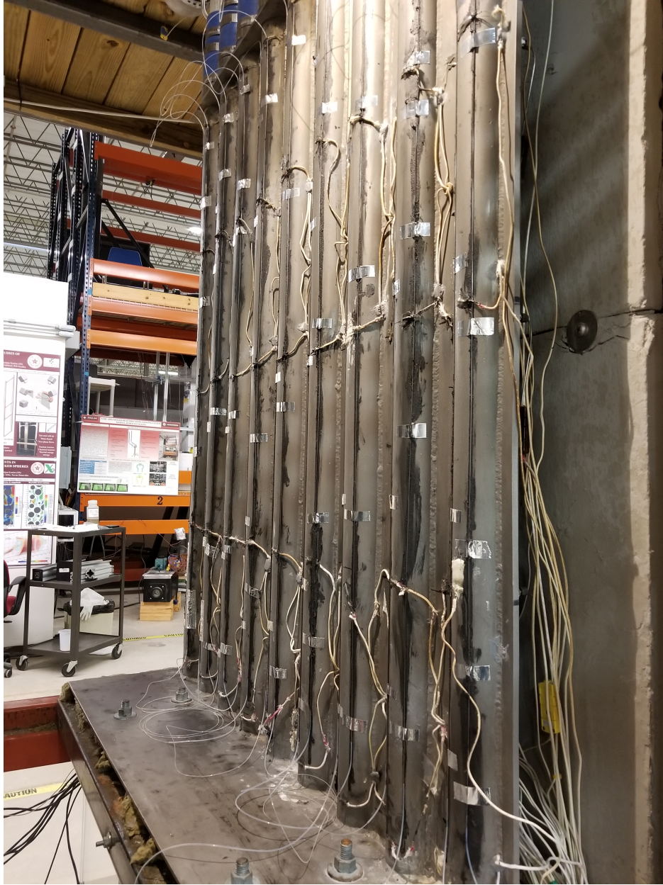
Figure 7.3: Full view of installed DTS on WRCCS cooling panel wall, first round of testing.
