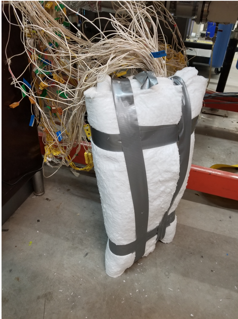
Figure 6.2: Method for obtaining room temperature calibration point for WRCCS thermocouples.
