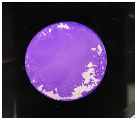
Figure 4.12 Membrane cracking problem caused by poor attachment when seeded by ENACT alone.
