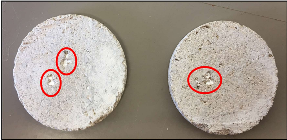
Figure 4-1: Two 4mm slices of a core after PLA injection Left: 2nd slice Right: 13th slice Reprinted with permission from (Shirley and Hill, 2019)
