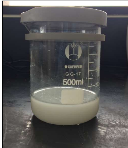
Figure 3-3: PLA in \text{CaCl}_2 brine suspension. Reprinted with permission from (Shirley and Hill, 2019)
