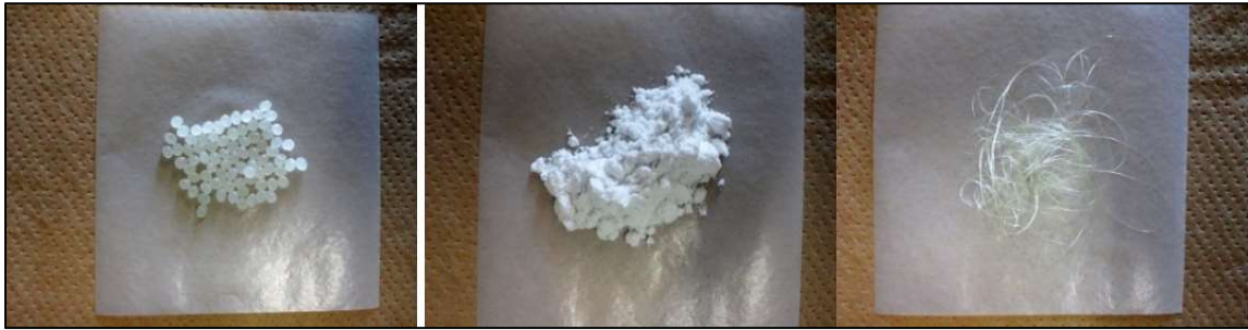
Figure 1-2: Different forms of PLA (Granular, Powder, and Fiber) (Adapted from Yoshimura et al., 2014)
