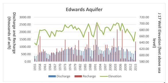
Figure 2: Edwards Aquifer Recharge and Discharge and the Elevation of J17 Well<sup>2</sup>
