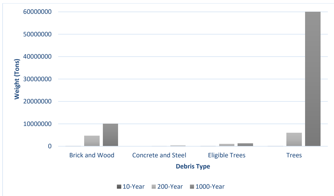
Figure 19: Debris expected from 10-year, 200-year, and 1000-year hurricanes
