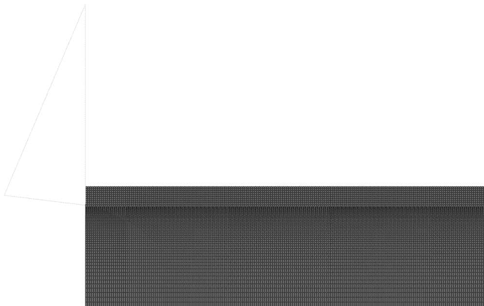
Figure 4-2. The initial model with the original mesh size, d = 0.01 mm
