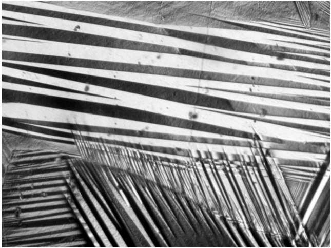
Figure 4.1.3 In-situ cooling experiment under OM reveals the thermoelastic martensitic transformation.
