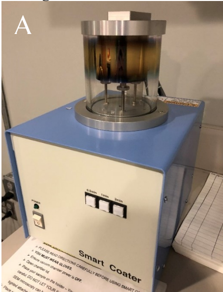
Figure 3. (A) Gold sputter coating machine and (B) mounted sample after sputter coating.
