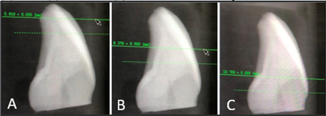
Figure 6. Microcomputed tomography scout scan selection of final scan area in the (A) incisal, (B) middle, and (C) cervical thirds of the sample.
