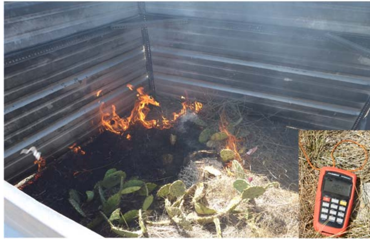
Figure 28. A view of a smoldering prickly pear cactus inside the burn compartment. The maximum fire temperature was measured with an OMEGA™ thermocouple sensor as the flames progressed through the plot consuming the succulent's photosynthetic tissue in a manner similar to that observed in Chapter IV.
