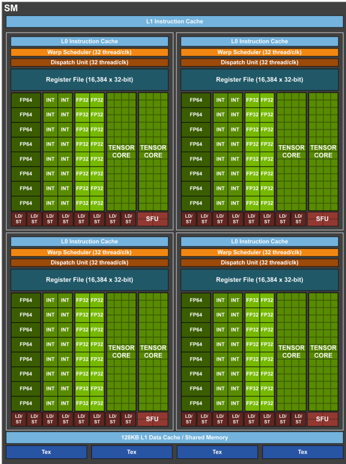
Figure 5.18: Core layout of the GV100 streaming multiprocessor.[32]
