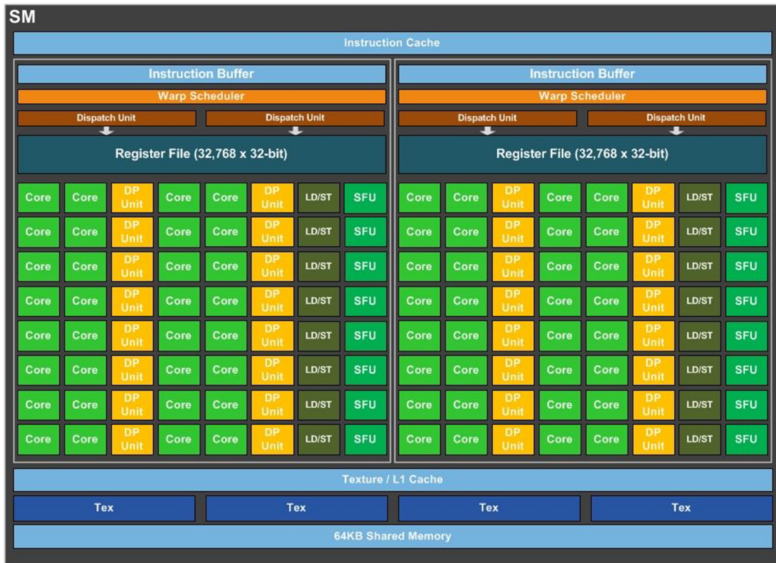
Figure 5.16: Core layout of the GP100 streaming multiprocessor.[31]
