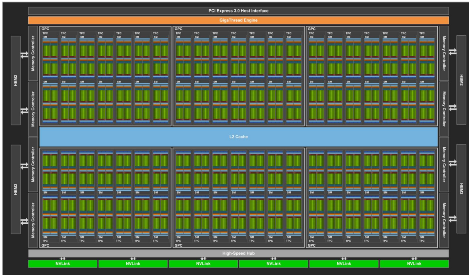
Figure 5.17: Streaming multiprocessor layout of the full GV100 GPU.[32]
