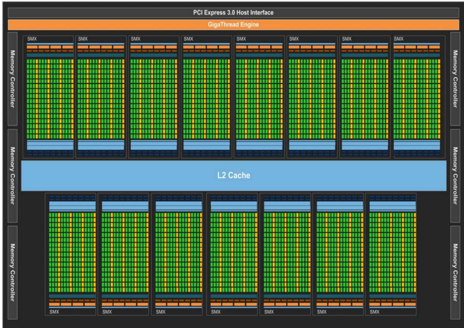
Figure 5.13: Streaming multiprocessor layout of the full GK110 GPU.[30]
