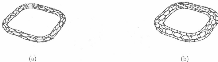
Figure 6. Fruchterman-Reingold 3D (FR3) NiceGraph drawings of (a) the toroidal polyhex with 120 hexagons and (b) the azulenoic cage with 10 pentagons, 100 hexagons and 10 heptagons.
