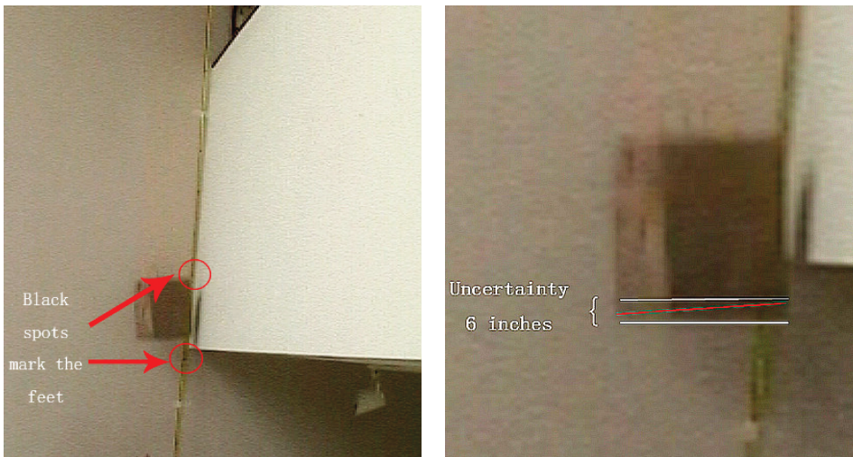
Fig. 3.2 Major sources of uncertainty in reading data. Left: blurred black marks on the tape measure indicating full feet (30.48 cm) of distance. Right: the error range in determining distances an object has fallen.
