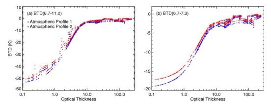
**Figure 18.** Changes in BTD along flight track relative to BTDs computed using sounding in Figure 3(b) for various scalings of the sounding's water vapor (WV). (a) BTD(6.7-11) and (b) BTD(6.7-7.3) for scaled WV above 7 km, (c) BTD(6.7-11) and (d) BTD(6.7-7.3) for scaled WV above 10 km.
