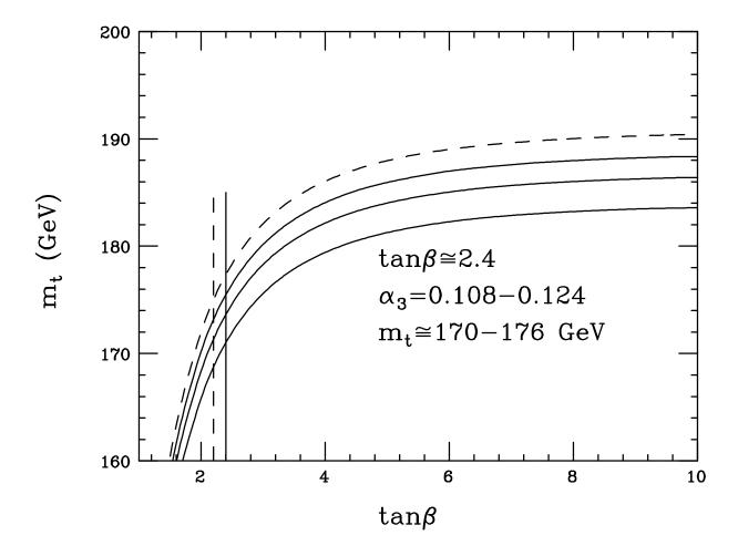
Figure 3: The calculated values of the top-quark mass as a function of  $\tan \beta$  for  $\alpha_s = 0.108, 0.118, 0.124$  (bottom,central,top solid lines) and  $M_U = 5 \times g \times 10^{17} \, \text{GeV}$ . Also shown (for  $\alpha_s = 0.118$ ) is the effect of taking  $M_U = 10^{18} \, \text{GeV}$  (dashed line). The vertical lines indicate the dynamically-determined value of  $\tan \beta$ . Note the stability of the  $m_t$  prediction.
