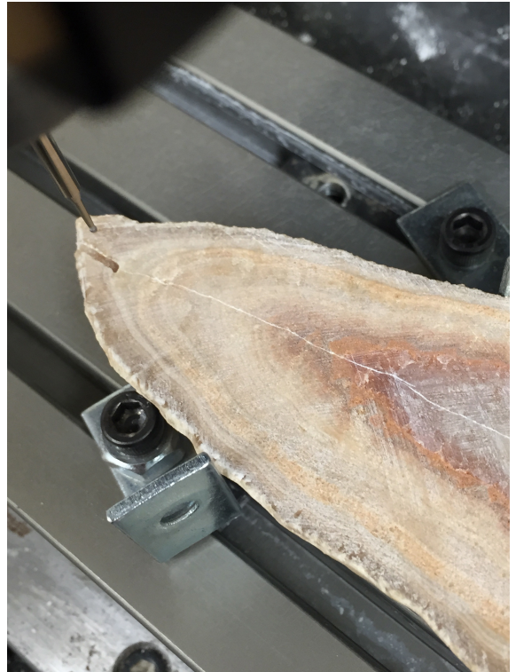
Figure 8- Micromilling a speleothem. A) View of the computer-controlled micromill. B) Up close view of milled speleothem
