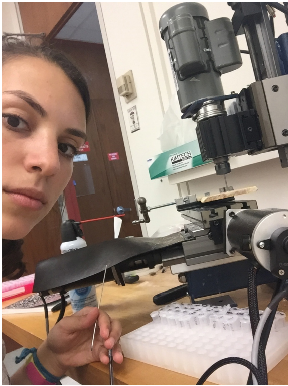
Figure 8- Micromilling a speleothem. A) View of the computer-controlled micromill. B) Up close view of milled speleothem
