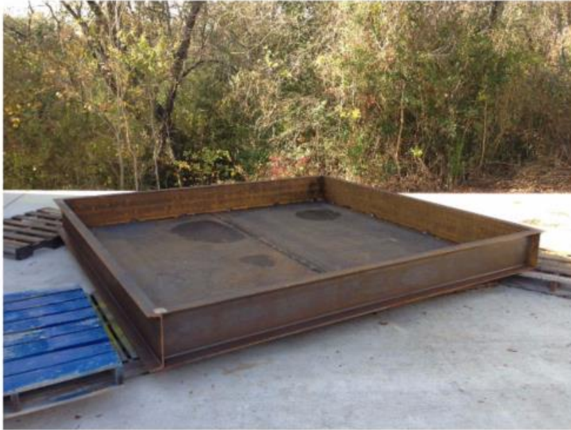
Figure 33: The testing tray that was constructed to contain liquid leakage.
