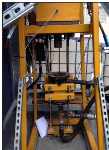
Figure 53: The testing chamber lowered to inspect the journal bearing
