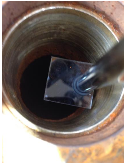
Figure 55: The borescope taking a picture of the bushing surface ID
