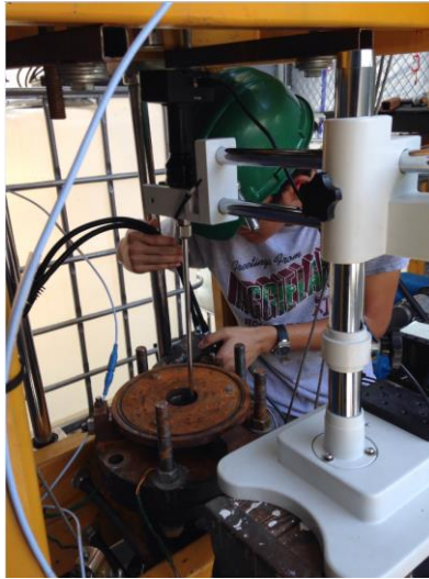
Figure 54: The borescope setup to take photographs of the bushing surface
