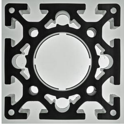
(a) Conventional lens setup normal to extruded aluminum rail
