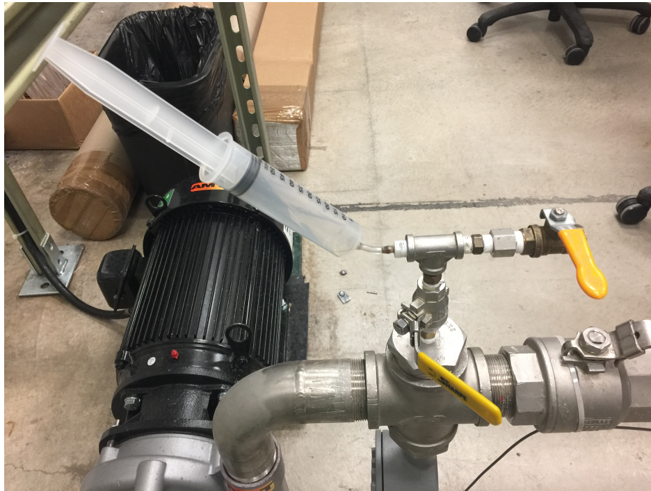
Figure 4.3: Seeding particle injection manifold can be operated with the facility online to ensure a well-mixed distribution and allow for real-time concentration control
