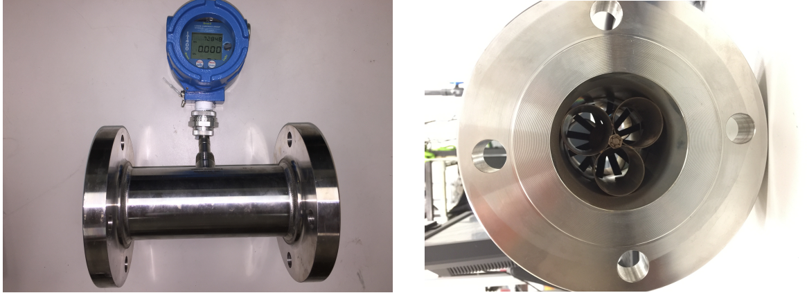
Figure 3.9: Sponsler SP3-MB-PHL-D-4X turbine flowmeter and IT 400 totalizer initially used to quantify the volumetric flow rate.
