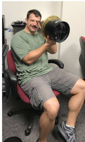
Figure 5.38: Edmund Optics TECHSPEC TitanTL model 34-012 mounted to the telecentric apparatus
