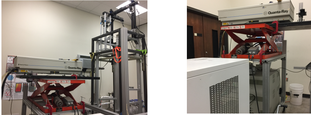
Figure 5.33: Mobile cart for the Spectra-Physics laser, controller, and air-cooled chiller
