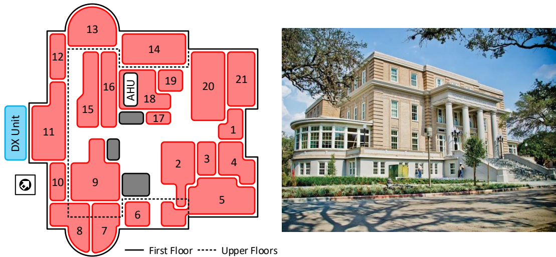
Figure 5.17: Basic layout of HVAC zones and exterior of the YMCA Building.
